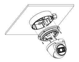
② Adjust the camera to obtain an optimum angle. Before adjustment, preview the image of the camera on a monitor. After that, tighten the set screw to finish the installation
